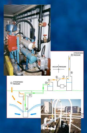
VEMPE has become the Technology of Choice for sites where it is desirable to extract both soil vapour and subsurface liquids
