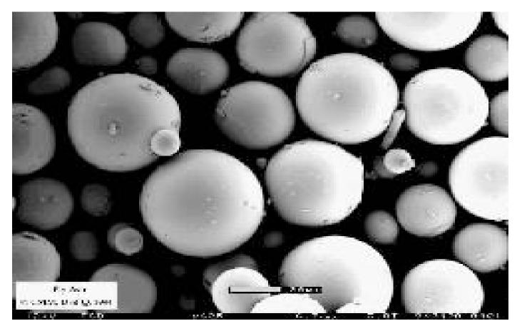
A pozzolan requires the presence of a reactive alumino-silicate glass. These glassy particulates must be fine enough to provide a sufficient reactive surface area for the solid-state chemical reactions. This reactive glass reacts with available calcium hydroxide and alkalies to produce cementitious compounds.(calcium-silicate hydrate gel and calcium-alumino silicates, etc.)
