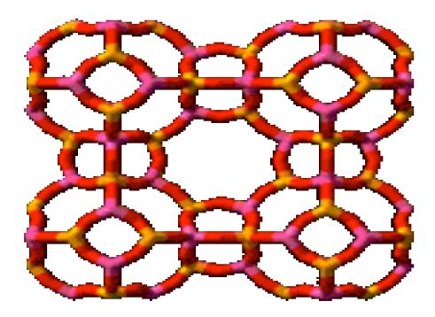
The pozzolanic channels (or pores) are microscopically small, and in fact, have molecular size dimensions such that they are often termed "molecular sieves". The size and shape of the channels have extraordinary effects on the properties of these materials for adsorption processes, and this property leads to their use in separation processes. Molecules can be separated via shape and size effects related to their possible orientation in the pore, or by differences in strength of adsorption.
